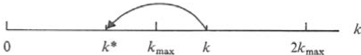
Figure 6.2 Misrepresentation of a wavenumber k > k_{\max} , in accordance with (6.4).
